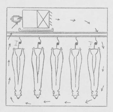
Fig. 2. Dry coil cooling room for pigs. Figures indicate air speeds in meter per second.
