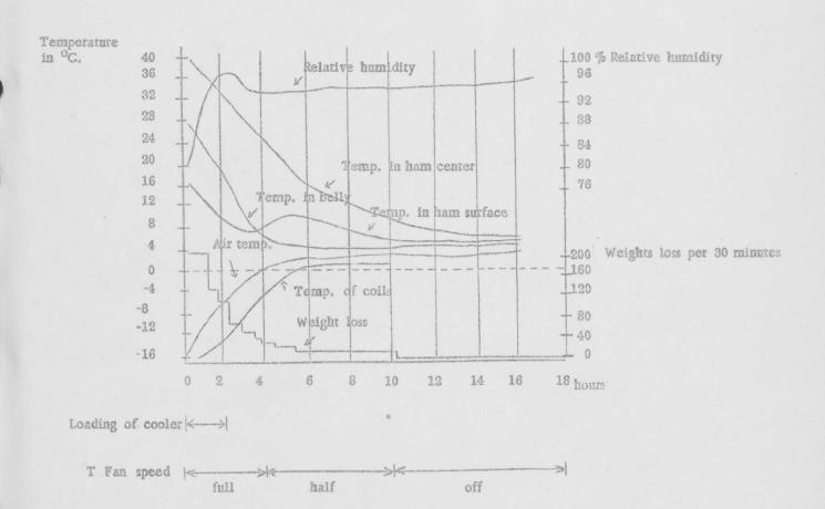
Fig. 1. Diagram of a quick cooling process for hog carcasses.
