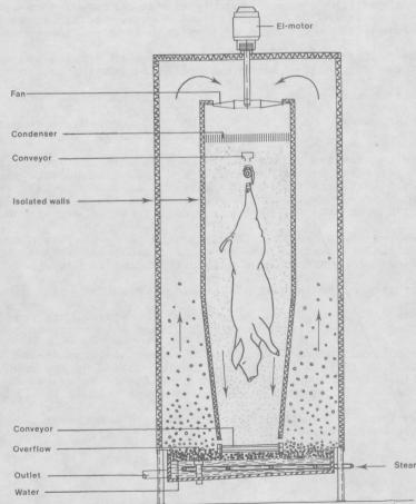
Fig. 1. Principle for scalding water With condensed water Vapor. (Meat Industry Technique AB, (MITAB), Malmö, Sweden).
