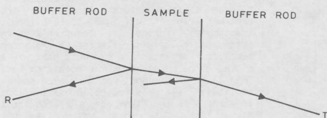
Fig. 3. The progress of an ultrasonic pulse from transmitter to receiver. At each interface part of the energy is reflected and part transmitted
