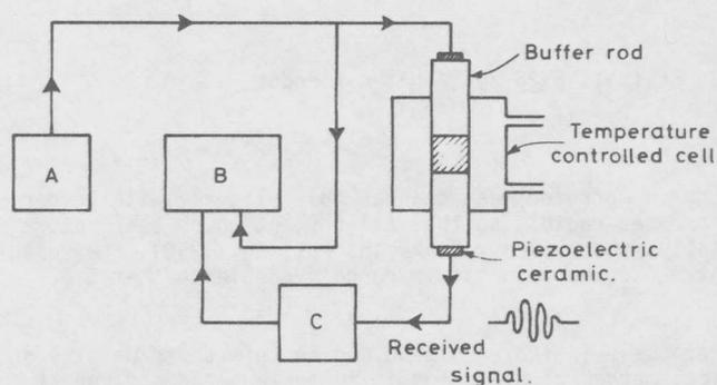
Fig. 2. Arrangement for generating and receiving electrical signals
