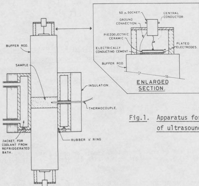
Fig.1. Apparatus for measuring the attenuation of ultrasound in frozen muscle
