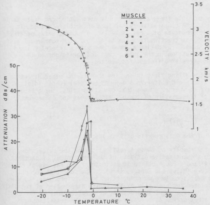
Fig.4. Attenuation and velocity\* of propagation of 2.25 MHz ultrasound along the fibres of beef *M. semitendinosus*
