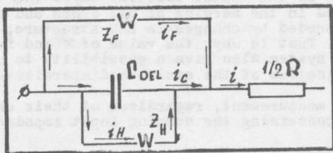
Fig. 2 Current circuits at the alternating current low-frequency impedansometry.
