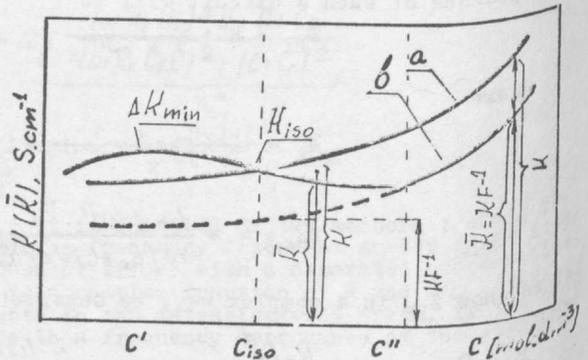
Fig. 6. Concentrational dependence of conductivity of a dispersion system, curve "a" and dispersion medium, curve "b".
