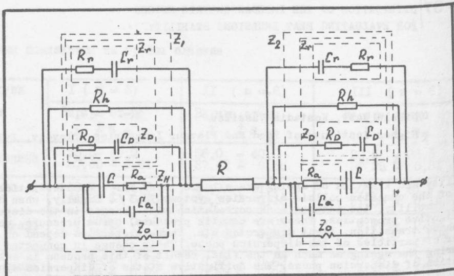
Fig. 1a. Equivalent electric circuit at low-frequency and conductivity measurement with a double-electrode cell, where,  $Z_1, Z_2$  - summing electrode impedances;  $R$  - ohmic resistance of the solution;  $C$  - DES capacity at the electrodes;  $Z_r, R_r, C_r$  - impedance and its component elements reporting the electrode reactive impedans <sup>D/11/</sup>;  $R_h$  a resistance of transmission.
