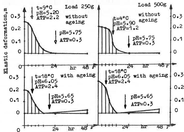
Fig. Elastic deformation resulting from stretching vacuum-packed hot meat during chilling.
