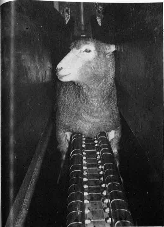
Figure 10. Sheep riding on the double restrainer system. Adjustable sides make it possible to handle animals weighing 23 kg (50 lbs.) to 227 kg (500 lbs.).
