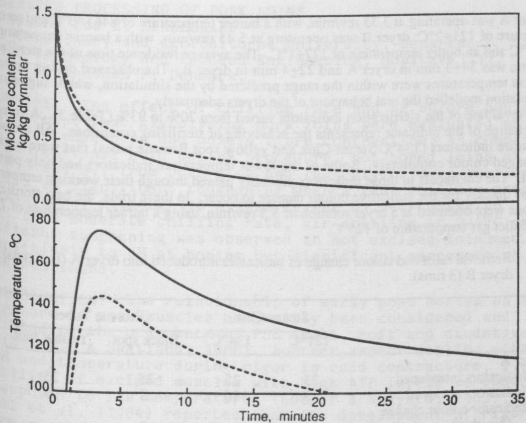
Figure 3. Simulated temperature and moisture profiles of 15 x 8 x 5 mm meal particles in a cascading rotary dryer. Particle inlet temperature 30°C; gas inlet temperature 700°C (--) and 800°C (—).
