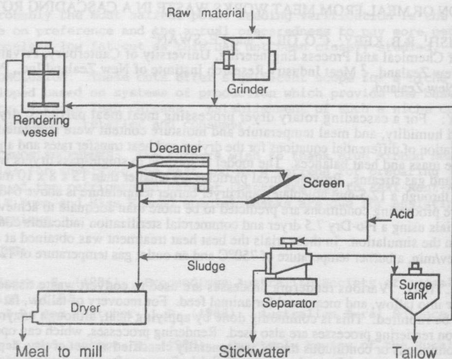
Figure 1. Schematic diagram of the MIRINZ low temperature rendering (MLTR) system.
