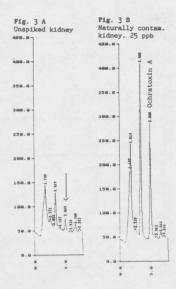
$0_{ ext{bv}iously}$  there is high background. This could be a natural background, or it could be caused by coeluting ponents. If it is a coeluting component it will probably not elute with the same retention time in systems with Other selectivity. For this reason tissue samples from different pigs and a standard of ochratoxin A dissolved the eluent are analyzed in 4 different systems.
