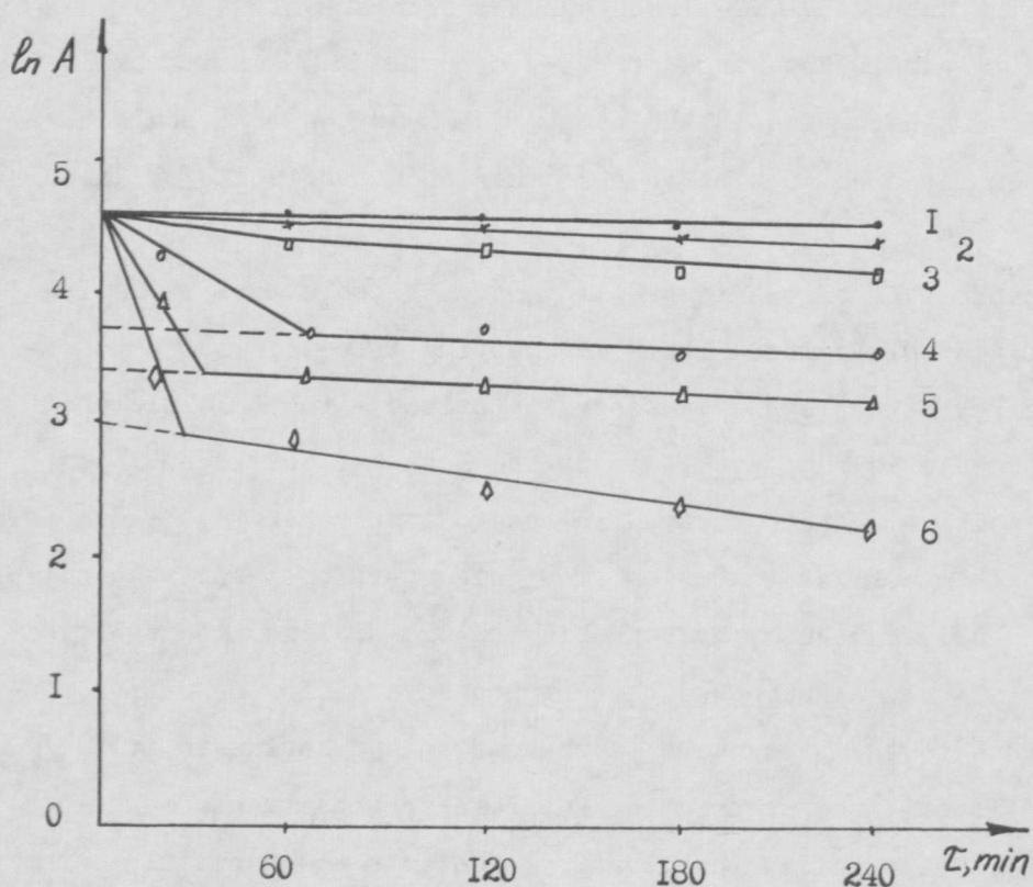
below 55°C for immobilized enzyme both fractions merge into some "mean" one with the corresponding mean inactivation constants. As seen from table 2, immobilization of pancreatin increases its thermostability by 1.5-3 times, and consequently, increases time of its action.
