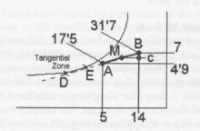
If we take the same air entering this new air treatment unit (this is: 14°C, 70% RH, h= 31,7 kJ/kg dry air, and an absolut humidity of 7 grs / kg dry air), it will leave the evaporator at 5°C and 90% RH (so h= 17,5 kJ/Kg dry air) and an absolut humidity of 4,9grs / kg dry air. On this way, the consumption is 31,7-17,5 = 14,2 kJ/kg dry air, but now it eliminates 7 - 4,9=2,1 grs of water / kg dry air. So, the energetic consumption we will have is:
