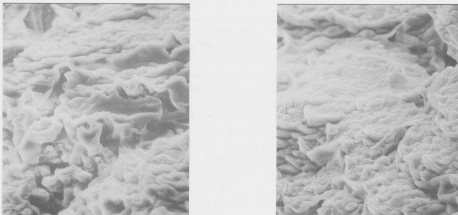
Figure 1. Scanning electron micrographs (400X) of non-retorted (left) and retorted (right) commercial frankfurters.
