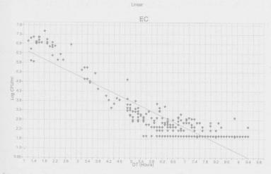
Calibration Code EC Active Data Points: 300 Specification Level: 1.00e+003 Cutoff Time (Hours): 5.37 Caution Time (Hours): 7.11
