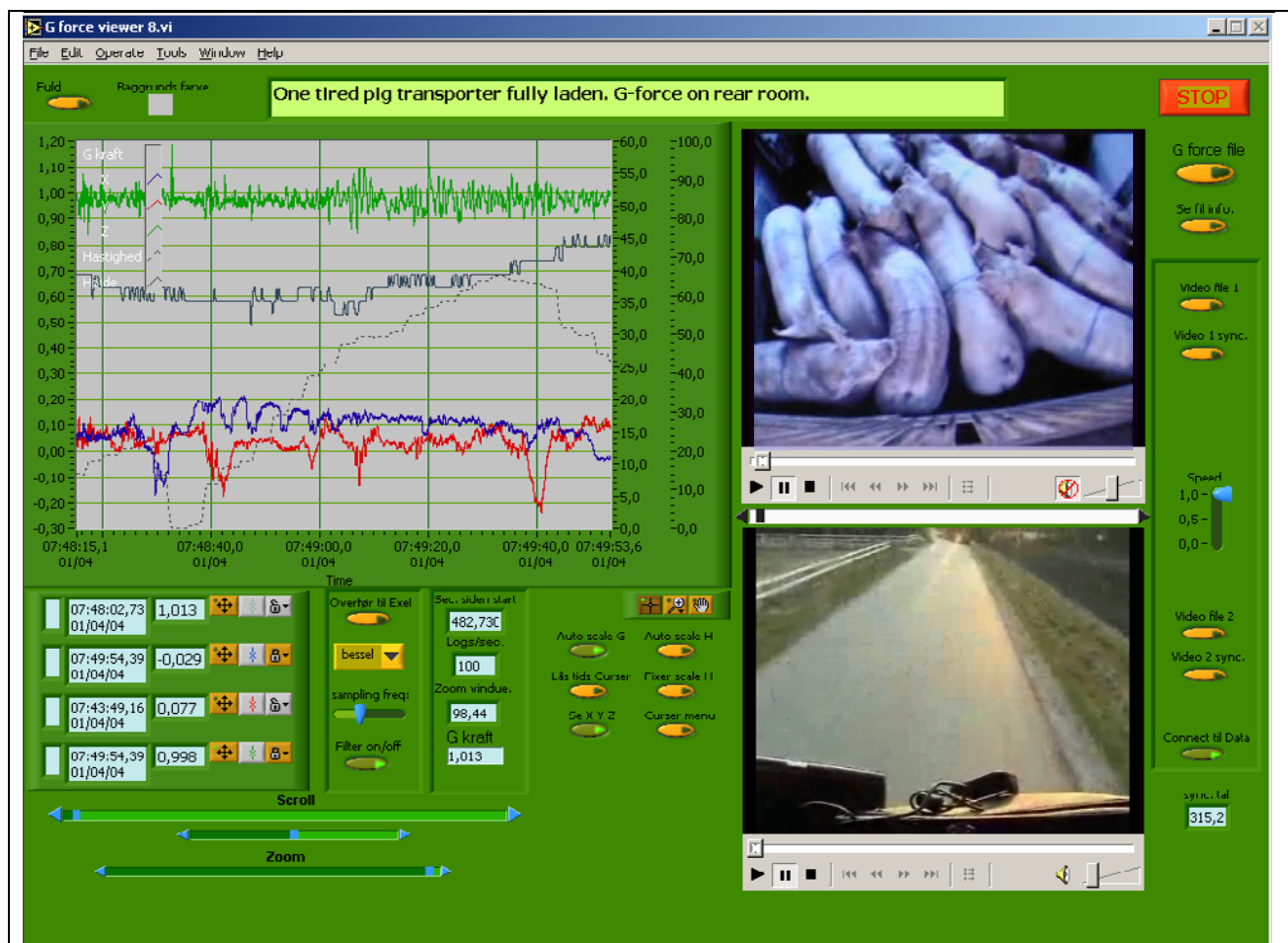
Figure 1. Screen display with two videos and graph showing curves for G-force in the x-, y-, and z-plane, vehicle speed, and altitude. The graph for the resultant force has been omitted for clarity. Data from rear pen. 1 st order Bessel low pass filtered.
