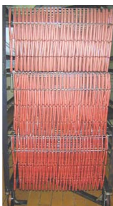
Fig. 3: Trolley with inhomogeneous dried sausages
