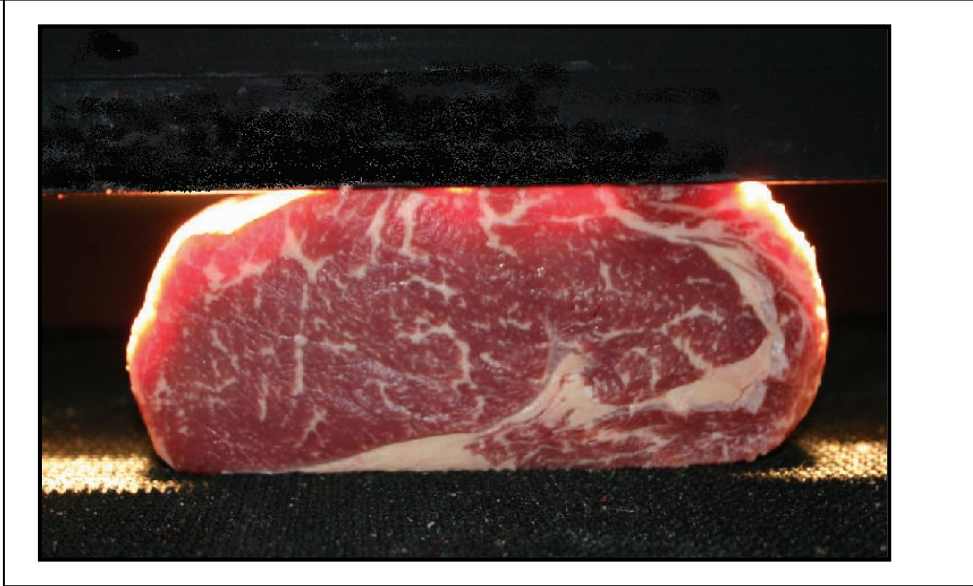
Figure 3. Entrecôte measurement from fat side (Titech Visionsort)
