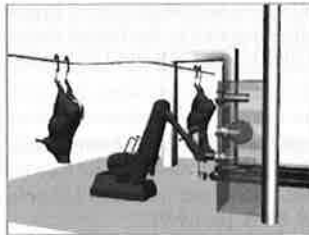
Figure 12: Automatic bung cutting, neck and breast opening, and removal of head and tail.
