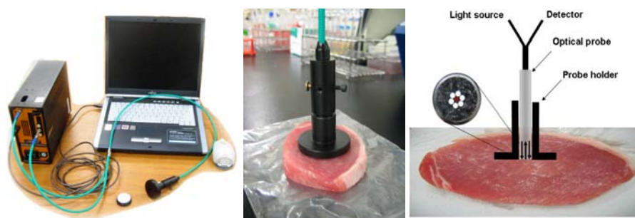
Figure 1. System of measuring NIR reflectance spectrum on pork loin.
