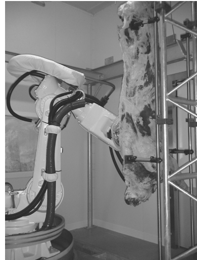
Figure 1: Robotic cell installed in the ADIV agro food pilot plant. A. Studied operation The studied beef carcass primal cut is a specific cut called 'Z-cut', which follows specific anatomical points on the carcass and leads to a forequarter with 5 ribs (AVT5) and a hindquarter with 8 ribs (ART8). The detail of anatomical points and the different cuts is illustrated in Fig. 2.
