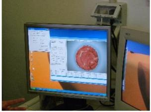
VIA system used in this study was inexpensive and suitable for wide use. It was composed of a video camera, a video light, an image analyzer, a monitor and a PC. Moreover colour and marbling were measured. Then steak was put in a plastic box (0.250 L) that was equipped with an active charcoal filter and tubes connected to PEN2 – Portable Electronic Nose (Airsense Analytics GmbH, Germany), (Fig. 2).
