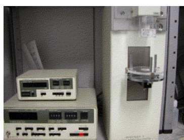
Fig. 3 Creep Meter used to measure rheological property examination.
