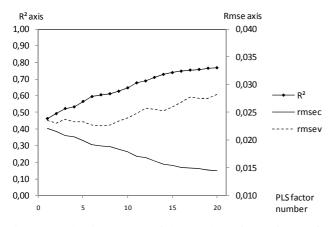
Figure 2: selection curves of the number of PLS factors for the loins cooking yield prediction by visible spectroscopy
