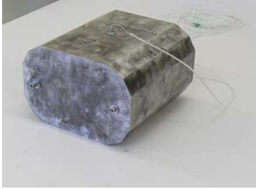
Fig. 2 Aluminium-made object having the same shape than a cooked pork ham
