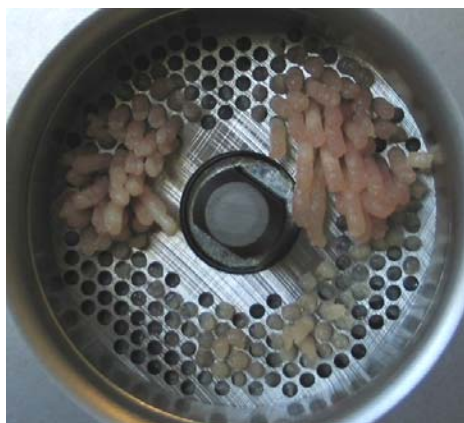
Fig.7: View of a grinder output (last plate). The differences in length of meat pieces are visible.
