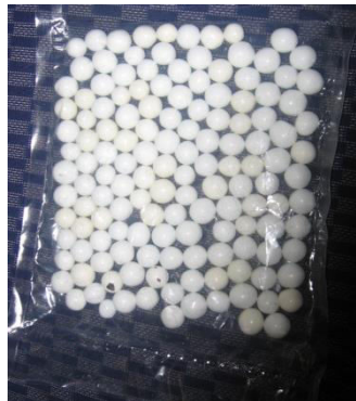
Heat sealed plastic swollen at altitude
