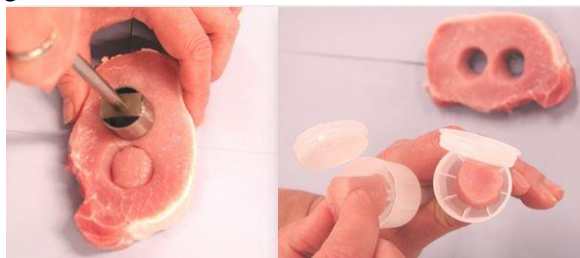
Figure 1. Preparation of samples for microwave measurements. A sample was taken from a slice of pork loin with a 25 mm diameter borer utilized to cut samples of meat. The meat sample was placed into polypropylene tube with a lid prior to measurement.
