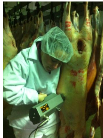
Figure 1. Measurement of a lamb carcass 25 min post slaughter using the GR probe.
