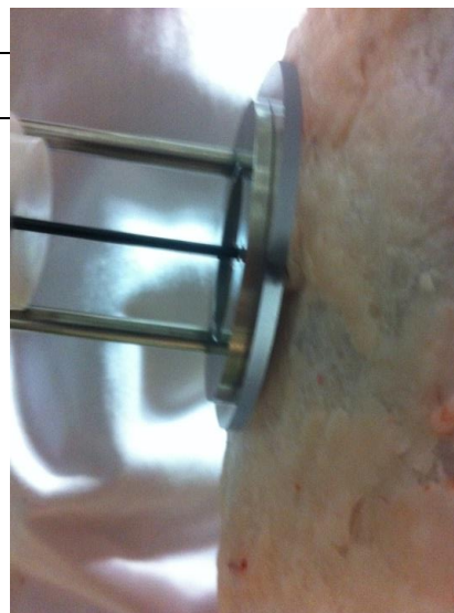
Figure 2. Measurement of a lamb carcass using the round plate on the GR probe highlighting the impact of carcass conformation.
