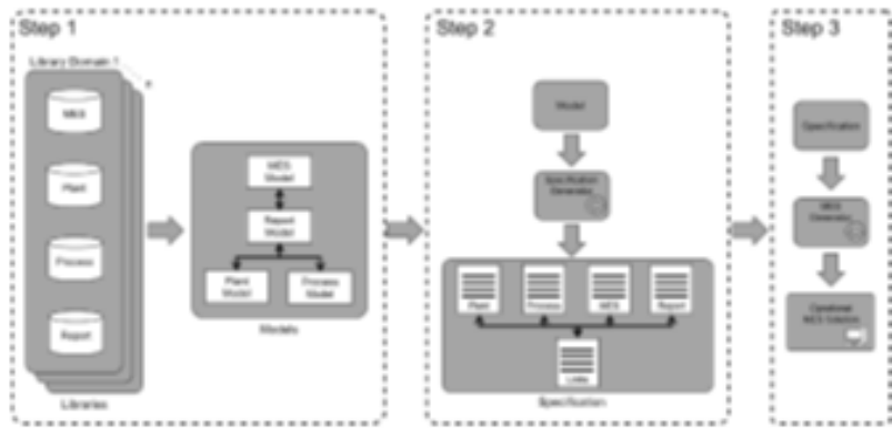
Figure 2: Overview of the model-driven approach for the automatic generation of MES.
