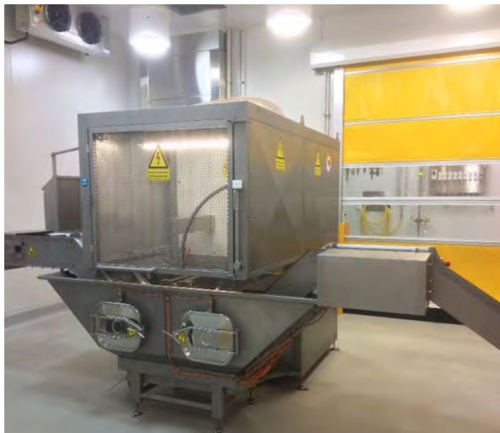
Figure 1. The Shockwave unit at CSIRO Coopers Plains, Brisbane used for this project
