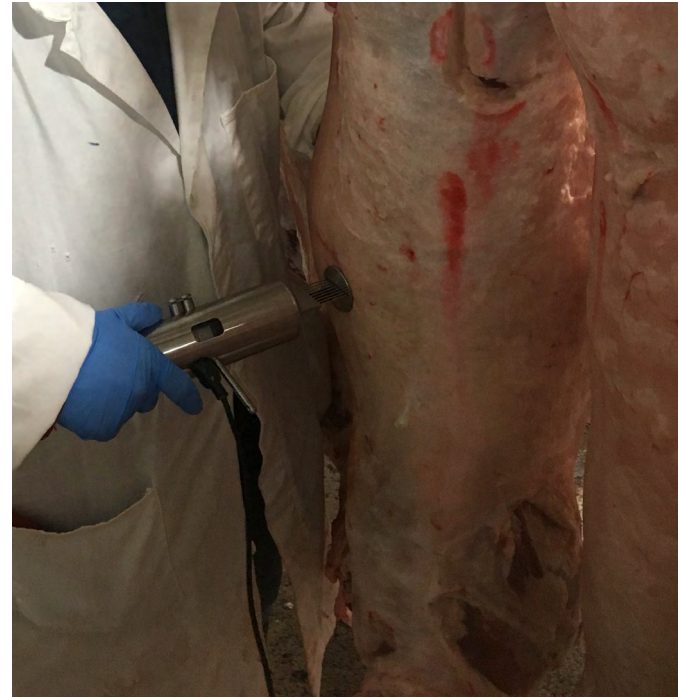
Figure 1. Measurement at the GR tissue depth site using the Icemeat probe .
