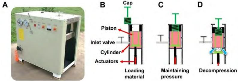
**Figure 1. The diagram of the SE process.** (A) The SE apparatus. (B) Raw material was loaded in the cylinder. (C) Steam pressurization phase, cylinder and piston were tightly coupled. (D) Instant catapult explosion phase, the piston was catapulted out of the cylinder, which was driven by the actuators and the kinetic energy of the steam and material.
