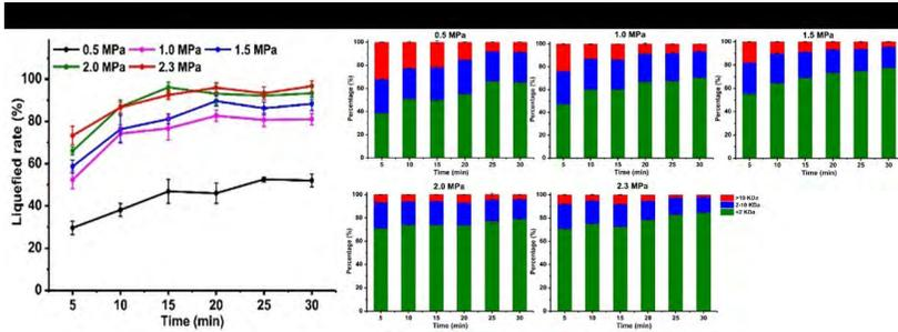
**Figure 3. Liquefaction of PHS by SE and the distribution of peptides in liquid fraction of PHS.** (A) The liquefied rate of different SE samples. (B) The distribution of peptides in liquid fraction of PHS
